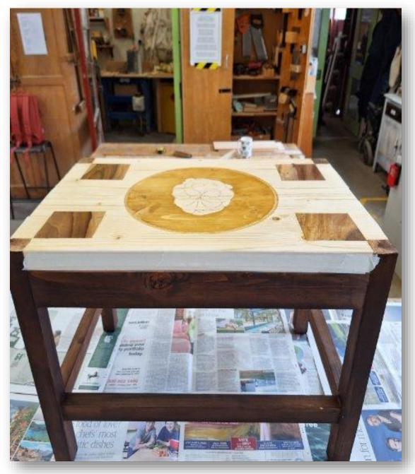
I used CLS wood to make the table, with mortise and tenon joints cut at a 45° angle so they meet at 90° this was for the framework whereas the tabletop was glued together and slotted on top with the 4 corners notched out. The inlay ended up being routed for the illusion because the CLS was not suited to cutting straight through. Finally, I gave all my wood a much-needed sanding and stained it walnut and antique pine for the insert and stencilled on a Pansie flower.
