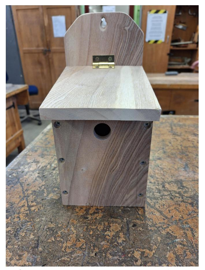
Simple but eye-catching design the lid is flush to the back board with a butt hinge and the bird box hang from the key shaped hole on a fence.
